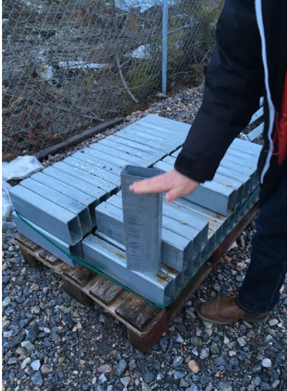
Socket which is inserted into asphalt (GEMS)
