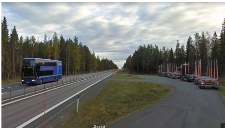
Figure 16: Pull-off Area on a 2+1 Road
